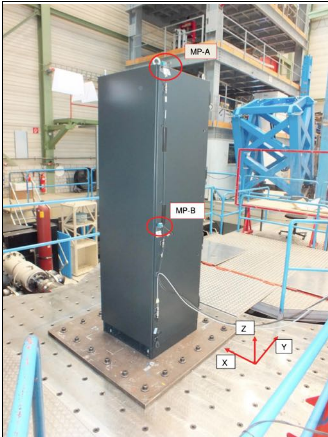
Fig. 23-5 Entire built-up for waveform testing (front)
