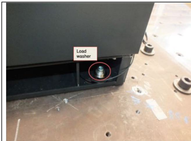
Fig. 23-3 Load washer application
