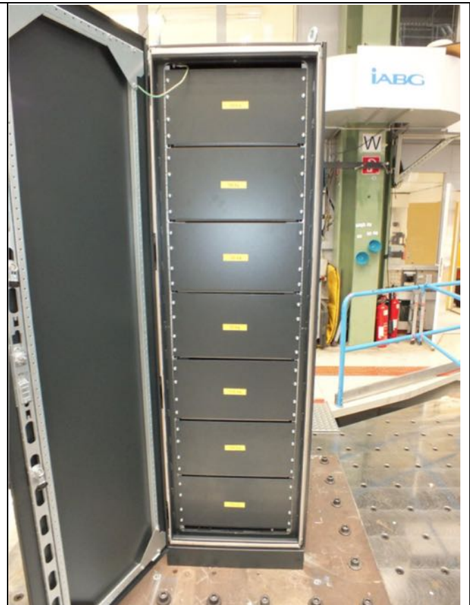
Fig. 23-6 The EUT with dummy weights
