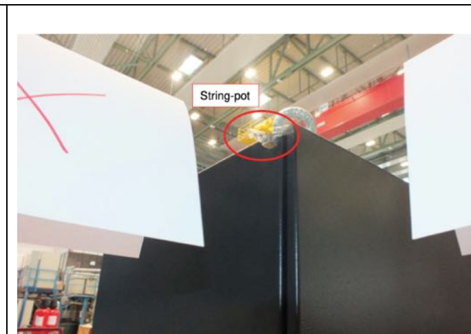
Fig. 23-4 String-Pot in X-Y directions to measure displacement
