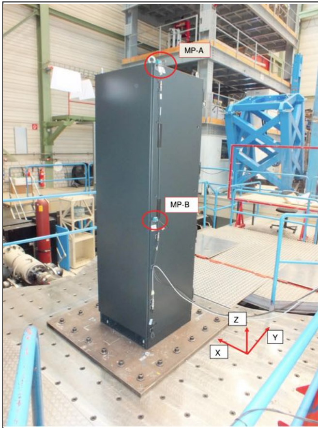
Fig. 23-1 Entire built-up for resonance search (front)
