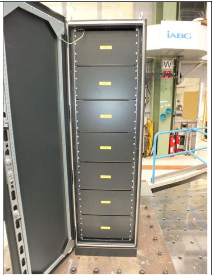
Fig. 23-2 The EUT with dummy weights
